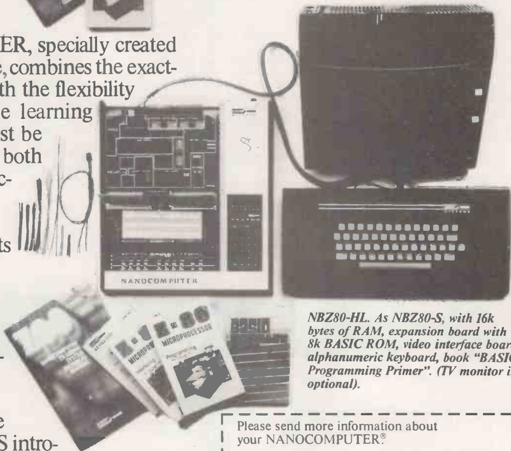
NBZ80-B. CPU board, keyboard, card frame/power supply, training book Vol. 1, Technical Manual.
